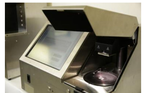
Figure 2: FITNIR Kappa analyzer/spectrometer showing the sample chamber.
