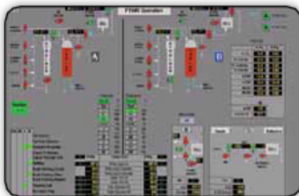
Figure 1: Operator's Graphic of the Canfor Northwood FITNIR/DCS System
